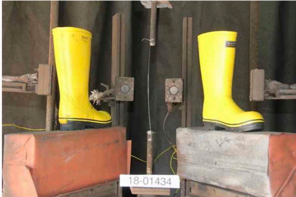
Figure 6-1: Boots as tested prior to arc exposure 18-01434
