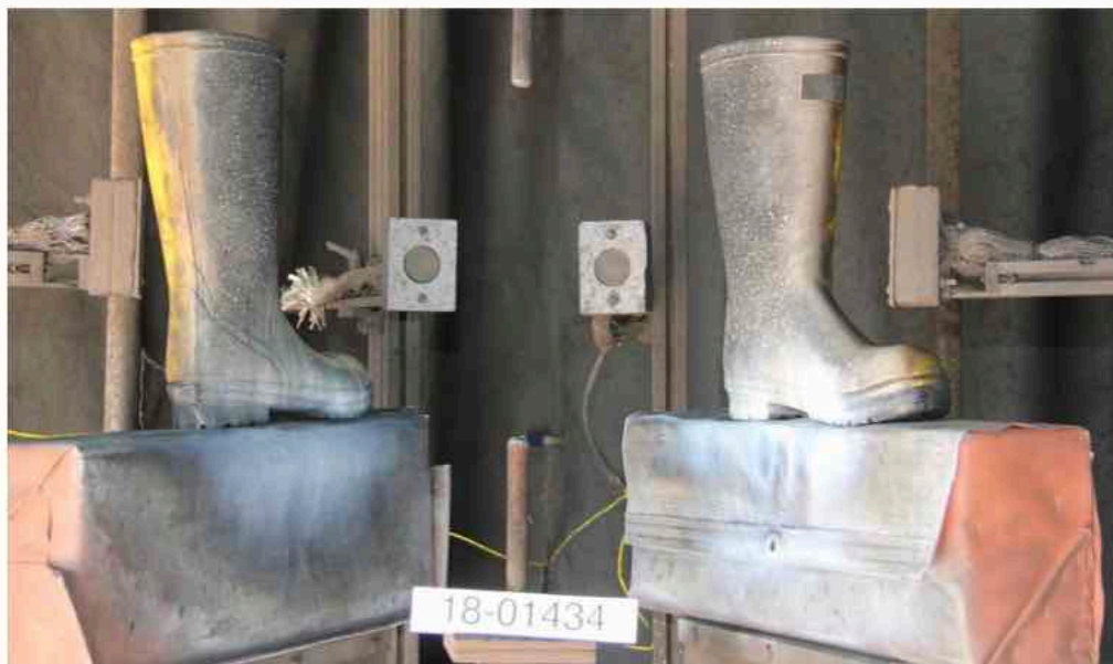
Figure 6-2: Boots as tested following arc exposure 18-01434
