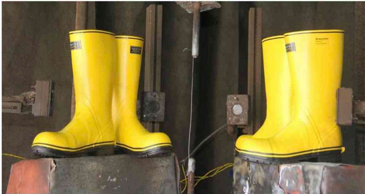
Figure 6-3: Boots as tested prior to arc exposure 18-2468
