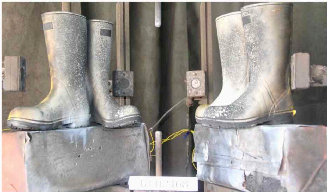
Figure 6-4: Boots as tested following arc exposure 18-2468
